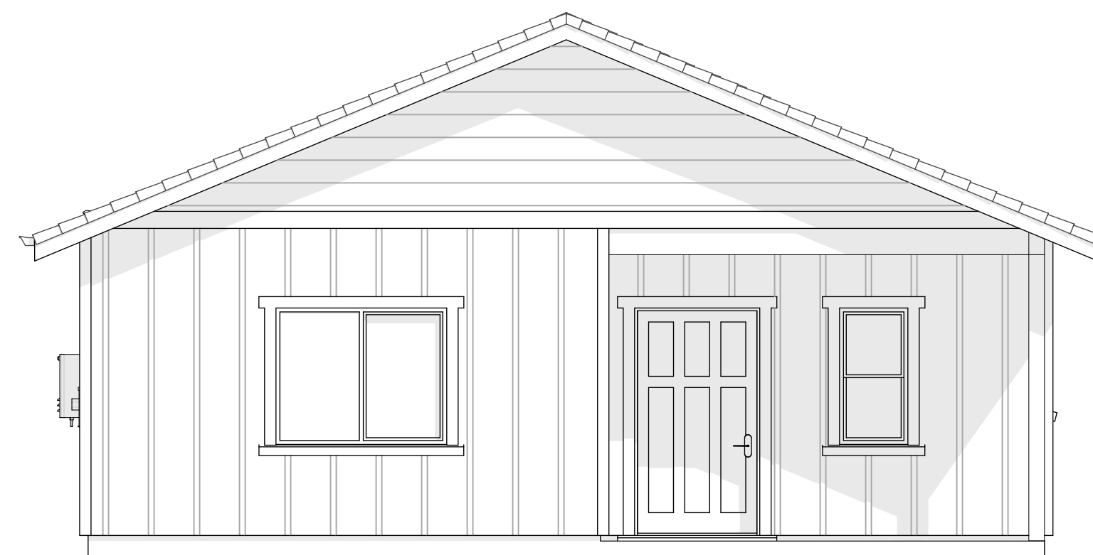
2 FRONT ELEVATION SCALE: 1/4" = 1'-0"
